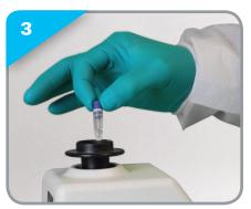
Replace the screw cap and mix by vortexing at high speed for 10 sec.
